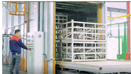
T6 Heat Treatment Furnace
